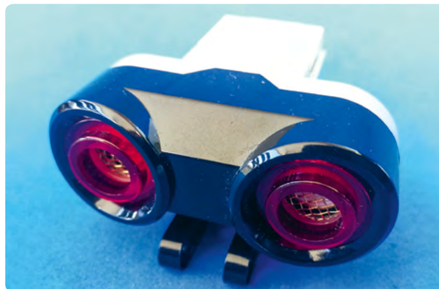
6: A LEGO ultrasonic sensor
