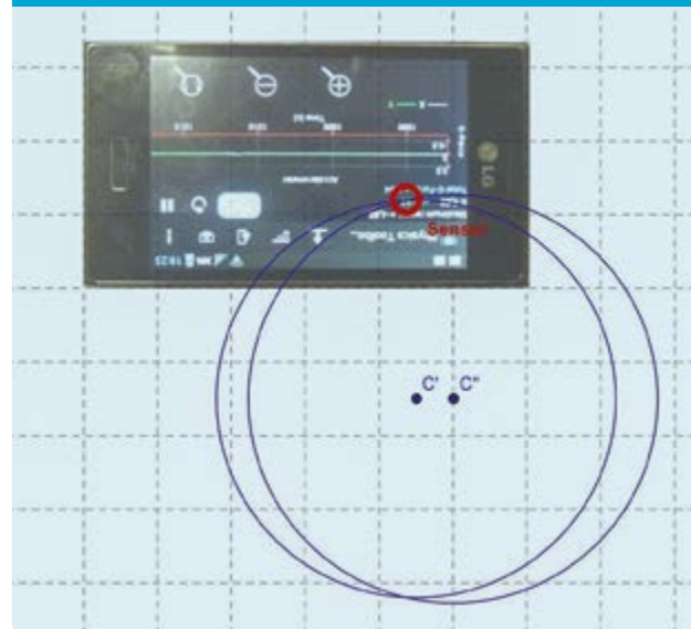
FIG. 5 The centres of rotation C' and C'' are the frames of reference for two positions of the smartphone on the record player
